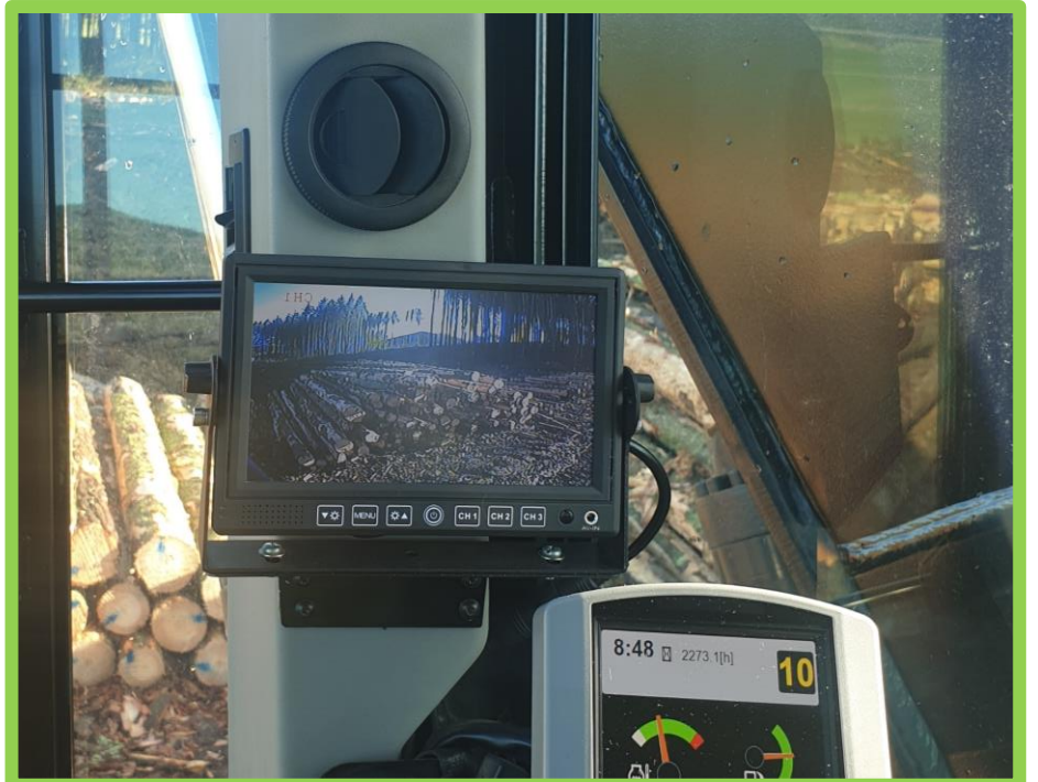
Photo 2: Screen in the cab to manage the risk created by the blind spot
