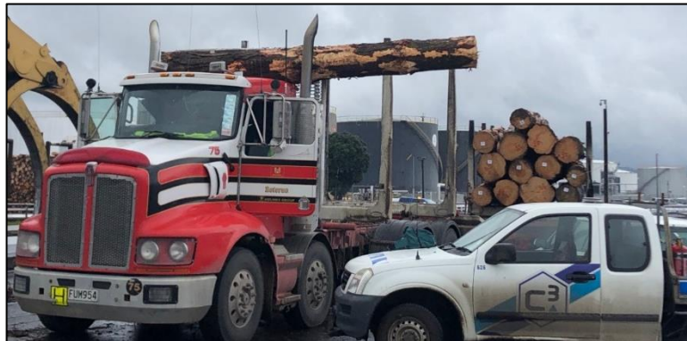
Picture 1 - Truck frontal view, post-incident, with the log wedged in place between cab guarding and exhaust.)
